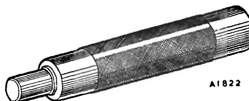
18G 589. First Motion Shaft Spigot Bearing Replacer
